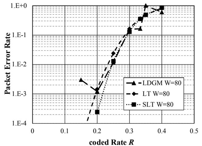
Fig. 6 PER performance versus code rate when interleaver length is  $N \times W = 1200 \times 80$  symbols.
