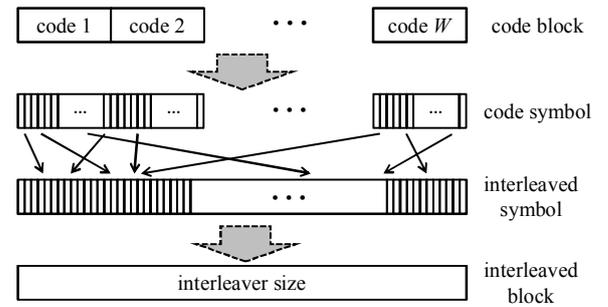
Fig. 2 Configuration of interleaver.
