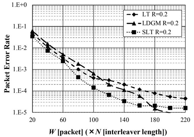
Fig. 4 PER performance versus number of codewords in interleaver.
