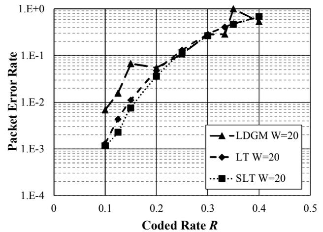
Fig. 5 PER performance versus code rate when interleaver length is  $N \times W = 1200 \times 20$  symbols.
