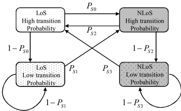
Fig. 1 Four state Markov model of downlink satellite-to-ground channel.
