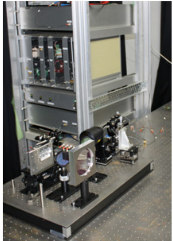
Fig. 2. Snap shot for experimental setup of an optical phase controller
