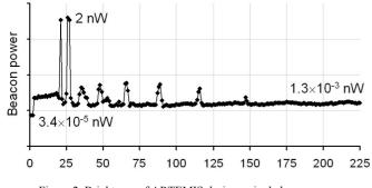
Figure 2. Brightness of ARTEMIS during a single beacon scan
