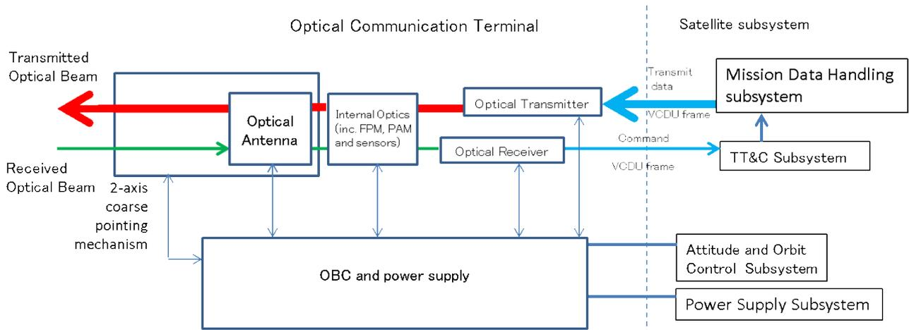
Fig. 1 Block diagram of the optical communication terminal
