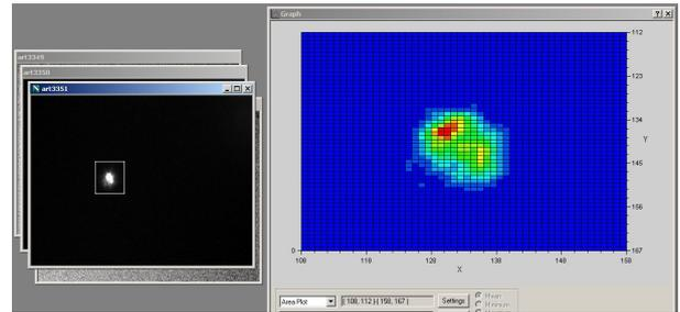
Figure 22. Image art 3351. ARTEMIS laser beacon beam via clouds
