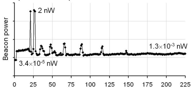
Figure 2. Brightness of ARTEMIS during a single beacon scan
